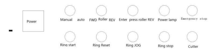
**POWER**: The main switch of machine power supply which is used to connect or shut off the machine power supply.
