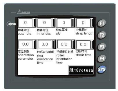
(1).Inner diameter of object: Input in actual size, with its unit as "mm".
