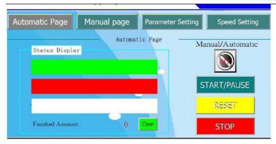
Automatic Page shows status dispaly ,finished amount and other manual functions. When machine work on the automatic model,
