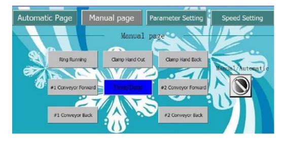
Manual page especially work for single pack or test machine before automation.
