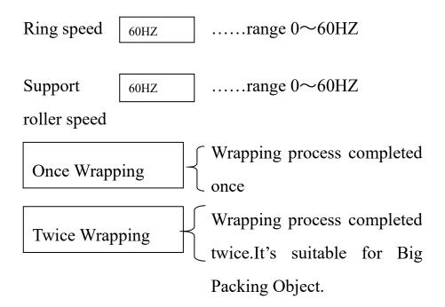
Note: • "Ring speed" and "Roller speed" not only define the running speed of ring and roller respectively, but are also in connection with the overlapping of packaging tape. The two setting parameters can be set by touching. If the ring speed is high and roller speed is low, the packaging tape features a large overlapping range; on the
