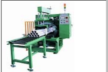
PVC Pipe Wrapping Machine The machine is special designed for Steel coil. The machine puts a tight and nice layer of film over all surfaces of the pipe.
