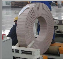
Steel Coil Packing Machine The machine is special designed for Steel coil. The package concept is an integral part of the coil packing machine design.
