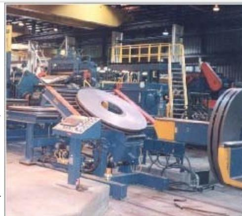
The package concept is an integral part of the coil packing machine design. The machine puts a tight layer of film over all surfaces of the coil. This tight layer of film eliminates most of the air from the package. By reducing the amount of air in the package, the potential for moisture to form is reduced, thereby reducing the possibility of corrosion or water spots.
