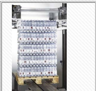
Stretch hood machine particularly palletizing and pallet packaging - play a critical role in safeguarding product in its highest value-added state for delivery to and use by customers
