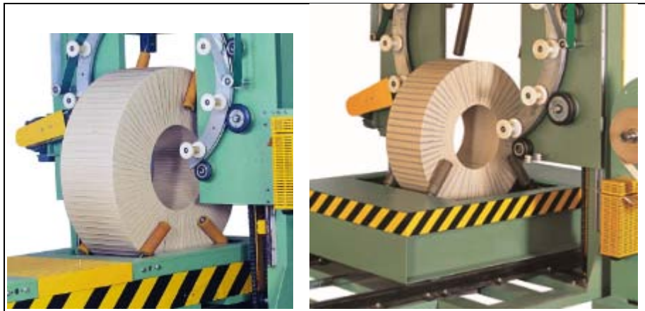
Coil packing machine with trolley for loading and unloading
